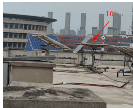
(b) 10^\circ angle of PV module experiment bench.
